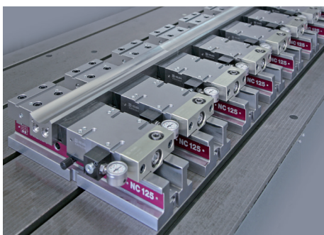
Workholding systems NC 125 with clamping force display
